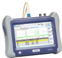
Handheld tester for fiber, 5G, Ethernet up to 100G, OTN, and legacy networks
