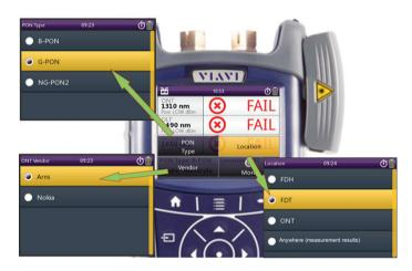
Easily select PON-type, Location, and Vendor to setup standard pass/fail thresholds providing reliable acceptance testing with simultaneous display of all PON and video power levels.
