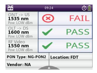
B/G-PON DS 1490 nm and US 1310 nm testingNG-PON2 DS 1600 nm and US 1535 nm windowRF-Video 1550 nm video overlay testing
